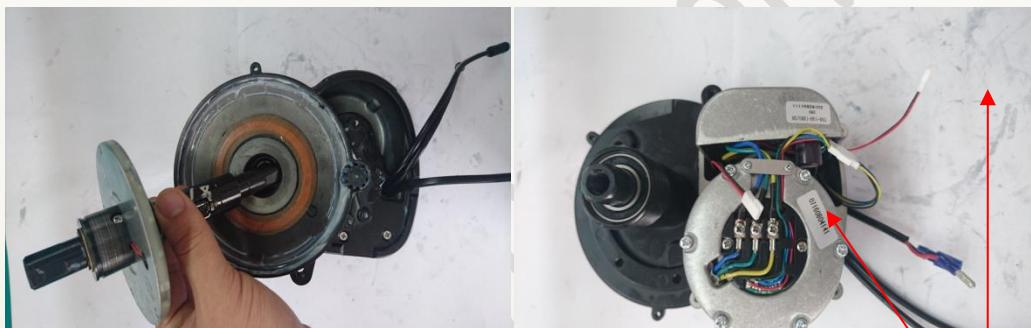
力矩与控制器连接线 torque sensor and connecting cable from controller
