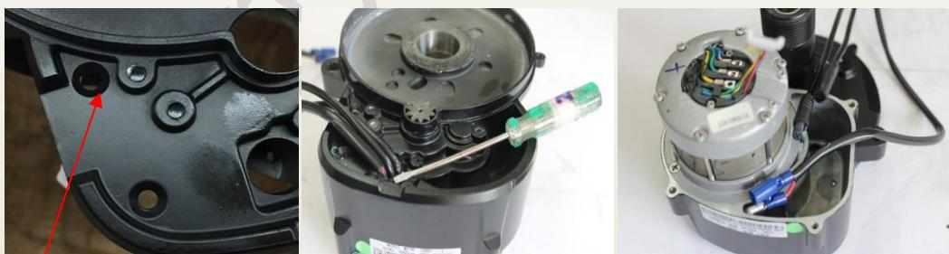
M3×6 螺钉孔位拆除线卡取出控制器及线卡 the position of M3×6, pull out the controller wiring harness
