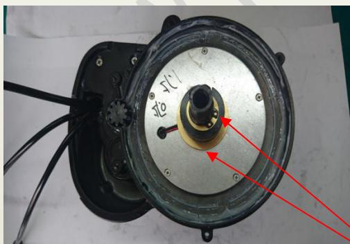
铜垫片及卡簧 copper gasket and circlip
