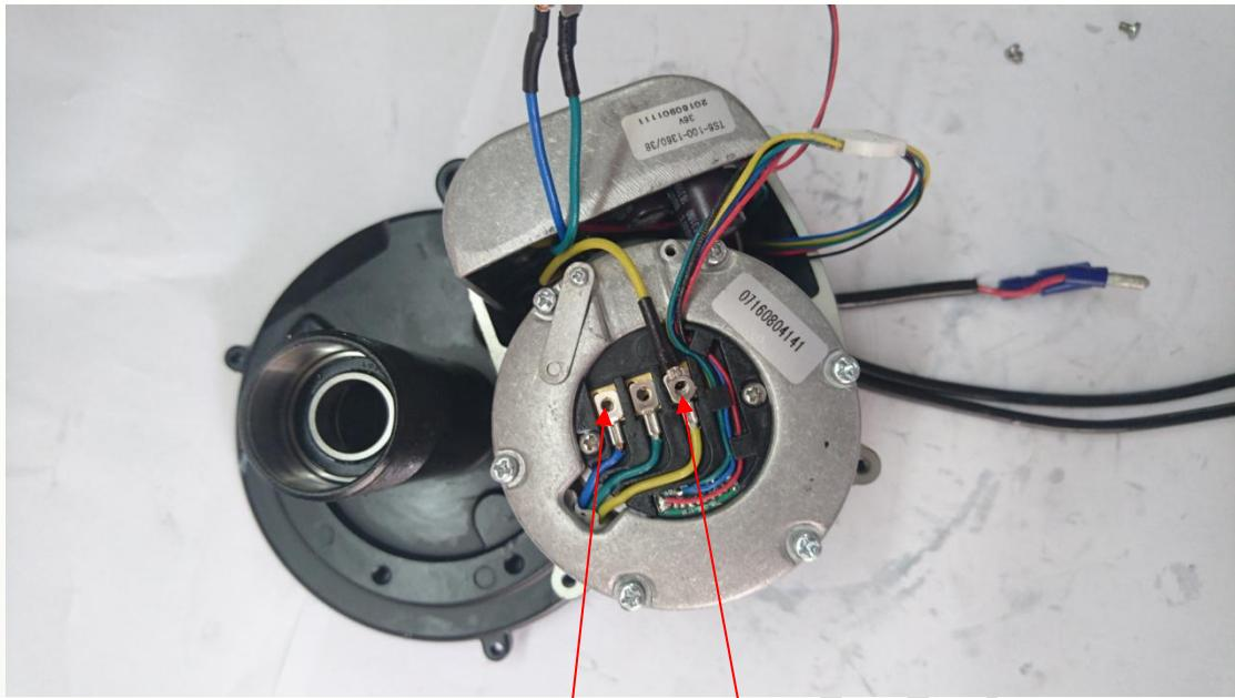
铆接焊片弹性垫片 riveting-welding chips
